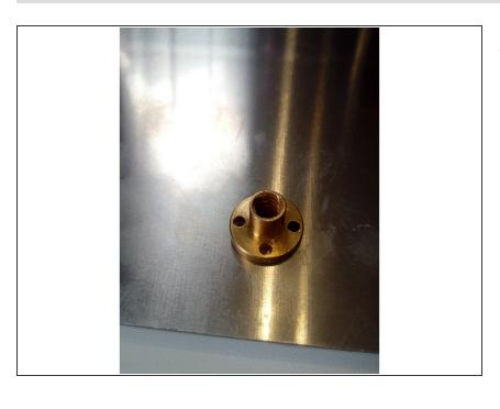
screw nut inserted from bottom
