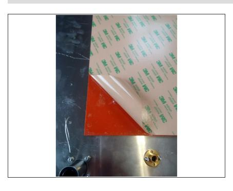
prepare the silicon pad. be carefull it's gluing very well
